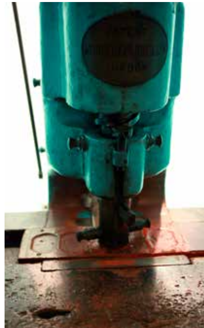
Old stamping machine used in the early 1970s.
